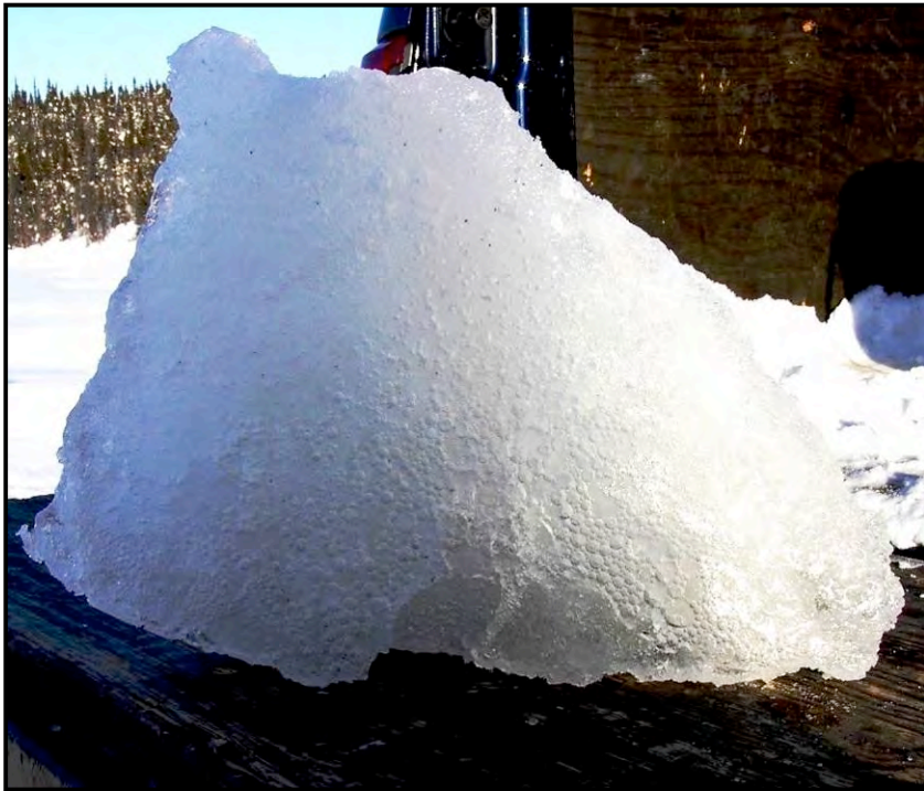
Poor ice quality showing high concentration of air bubbles
