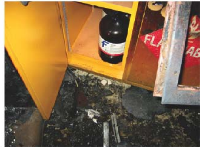
Flammable solvents inside were protected from the fire
