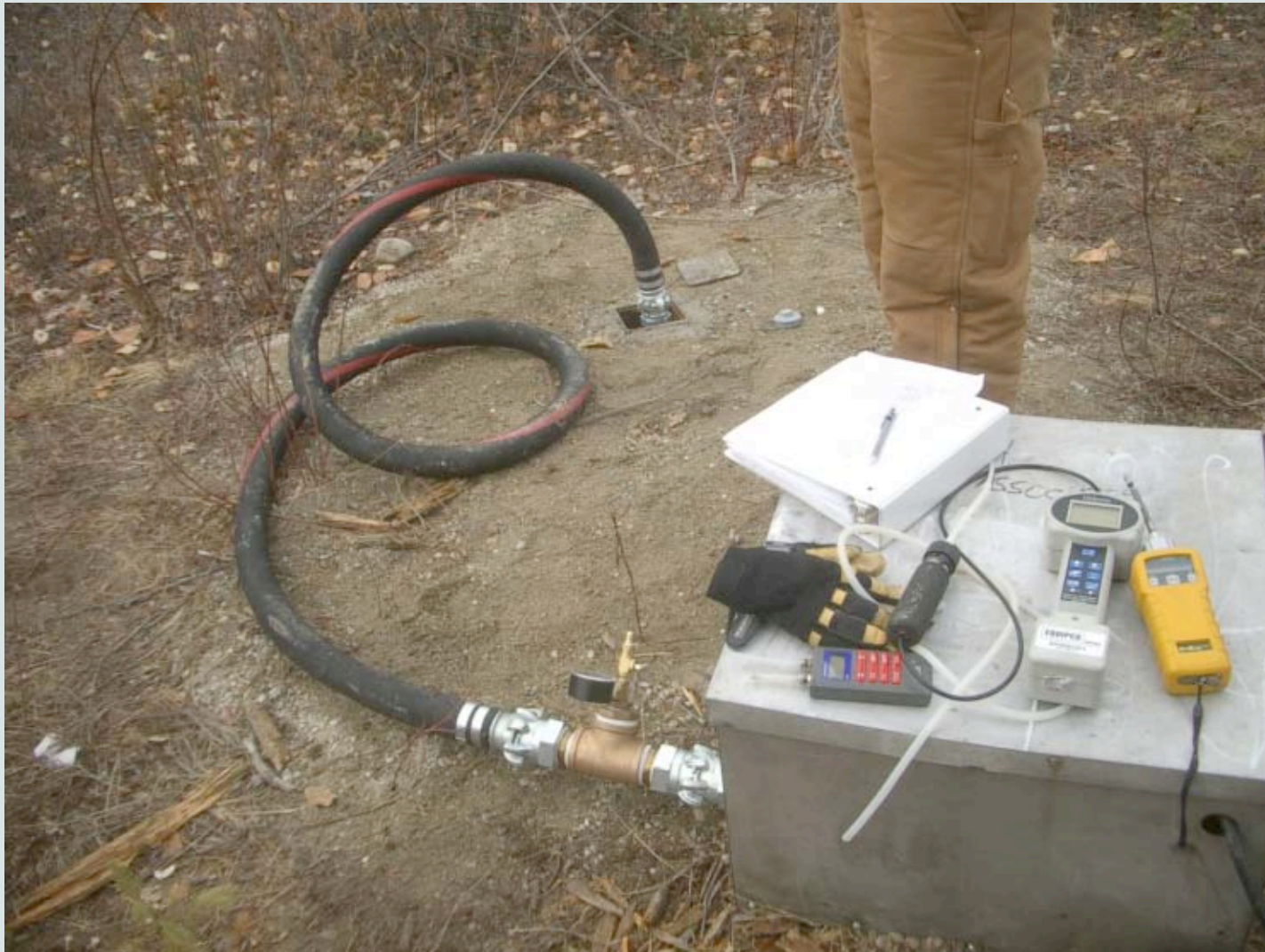
Simple Bioventing Pilot Test
